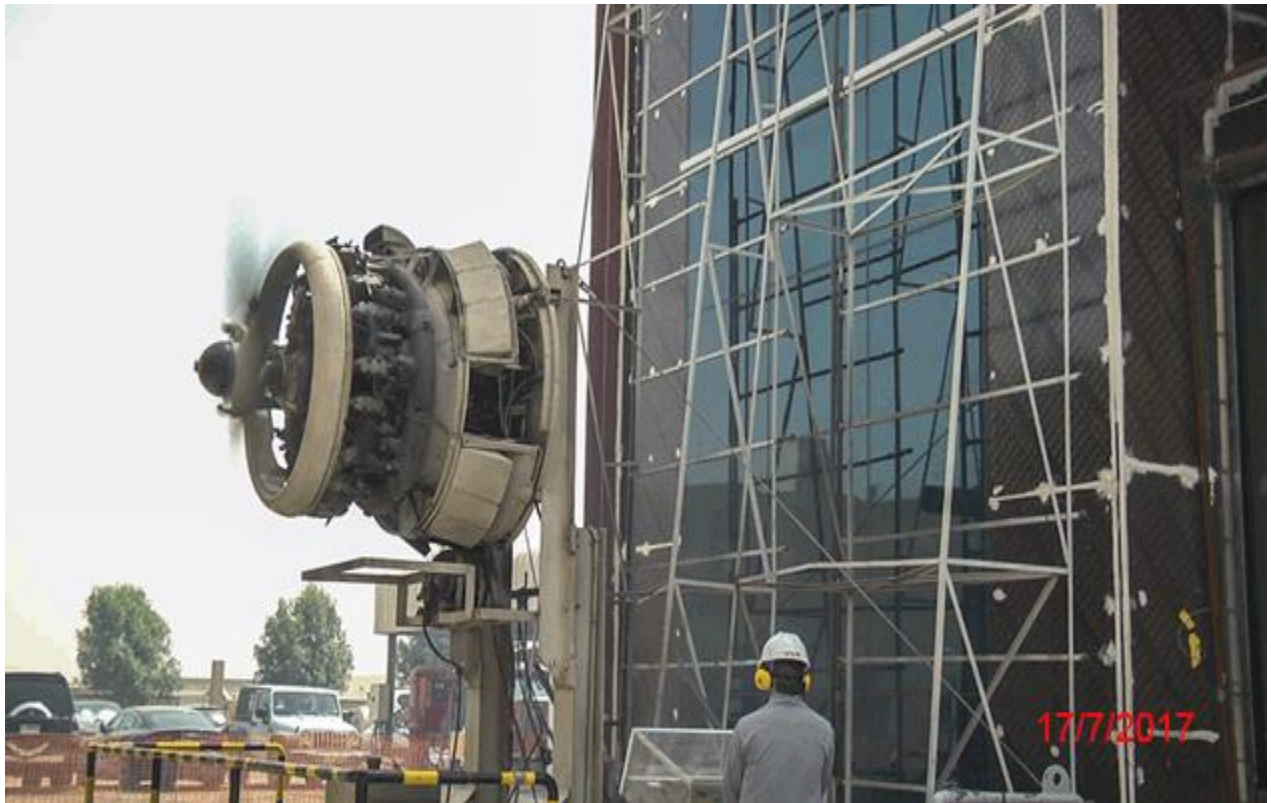
Dynamic Water Penetration Test
